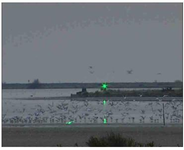
In 2000, a prototype of automatic system scanning the runways with a low low height laser beam is developed in France. The beam's specifications guarantee a complete ocular safety for both ground staff and cabin crew.
