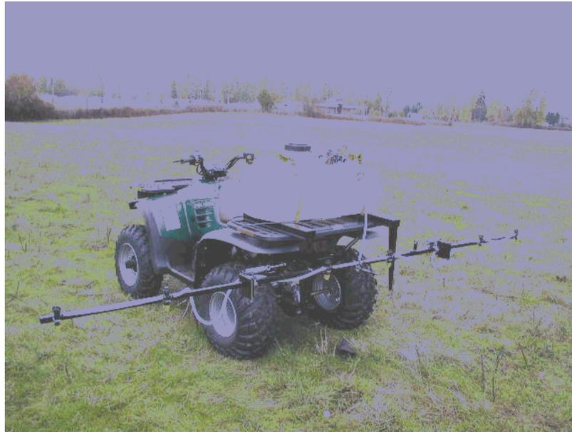
*Figure4 - An example of an All Terrain Vehicle (ATV) modified with a boom sprayer and a mixing tank. This system was used for the Flight Control® test at Portland Intl. Airport.*
