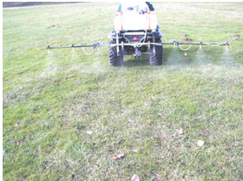
*Figure5 - Example of a turf application of Flight Control® using a boom sprayer and fine atomization.*
