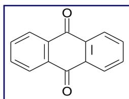
Figure 1. The Chemical Structure of Anthraquinone,  $C_{14}H_8O_2$ .
