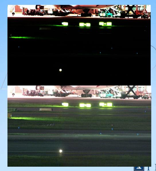
Images from Stratech Systems Ltd iFerret FOD detection system
