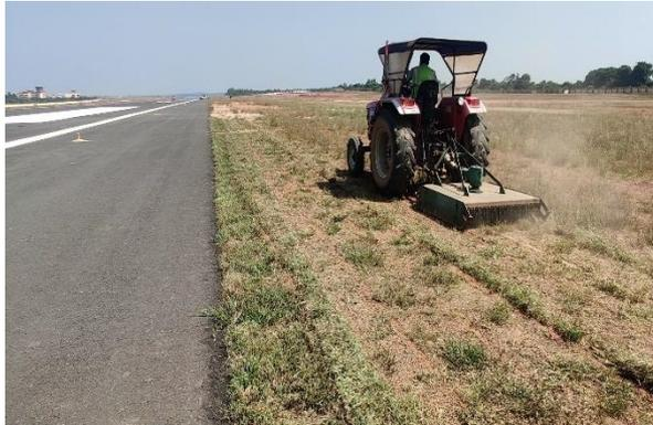
Grass Cutting Machine deployed for control on RWY Strip.
