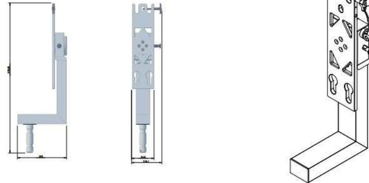
Tripod holder with Quick-Lock quick-release Fastener for one AHD-215X systems
